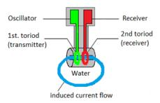
Both toroid cores are flowed through by the medium to be measured.
