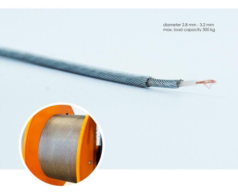
The two-layer stainless steel cable with insulated inner conductor has a comparatively very high load capacity with a small outer diameter. With a modulation method such as FSK or Powerline, the voltage supply and data transmission of oceanographic or limnological water measurement devices can be performed simultaneously.
