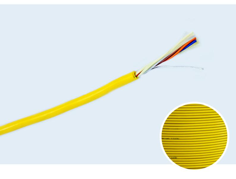
Rugged multicore cable for continuous underwater use in fresh- or seawater. The Jacket is made out of very abrasion und cut through resistant polyurethane. The four conductor cable can be used for simultaneous supply and data communication e.g. via RS-232 or RS-485 used for the electrical connection of oceanographic or limnological water measurement devices.
