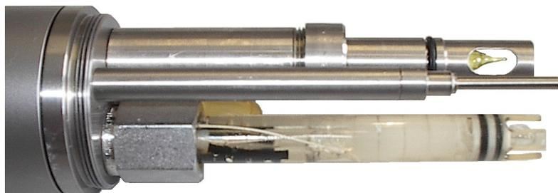
Probe with removed protection cage. Sensors for H<sub>2</sub>S, pH, temperature and depth.
